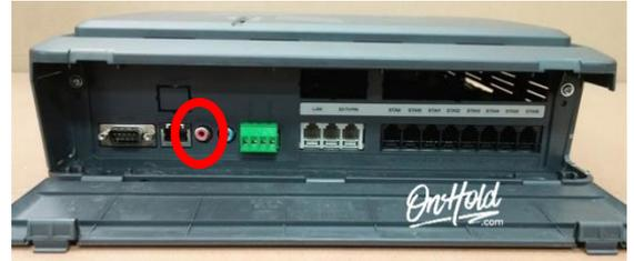
The other end of the audio cable will connect to the back of the on hold player, to the 600Ω output.
