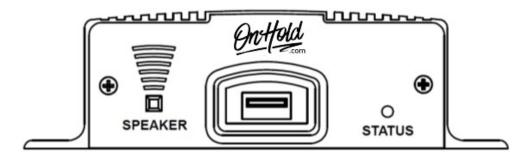
SPEAKER - The SPEAKER switch can be turned ON and OFF to monitor music on hold audio playback. The switch has no effect on the audio output connections on the rear of the unit. Switch should normally be kept OFF. (NOTE: The SPEAKER volume is fixed and is independent of the Volume control on the back of the unit.)
