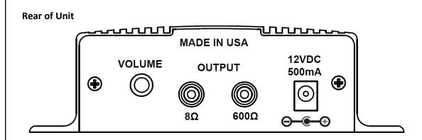
VOLUME - This pot is used to control the  $8\Omega$  and  $600\Omega$  output level of the stored messages. Volume up is clockwise, volume down is counter-clockwise.
