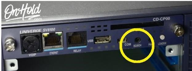
On the cabinet is a port labeled “BG/MOH”– this is where you’ll connect the on hold player. The on hold player includes an audio cable and a small adapter piece. You may need to connect the adapter piece to one end of the audio cable if the audio cable does
