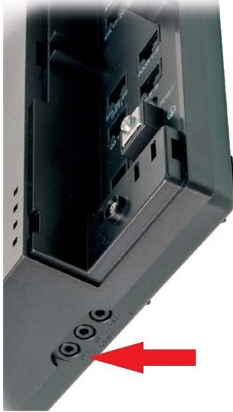
On the bottom of the cabinet is a port labeled “Audio1” – this is where you’ll connect the on hold player. The on hold player includes an audio cable and a small adapter piece. You’ll need to connect the adapter piece to one end of the audio cable, which will then connect to the “Audio1” port on the phone system. The other end of the audio cable will connect to the back of the on hold player, to the 600Ω output.
