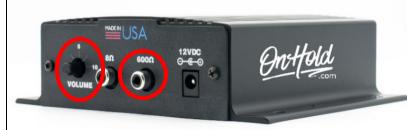
connect the adapter piece to one end of the audio cable, which will then connect to the "AUDIO" port on the phone system. The other end of the audio cable will connect to the back of the on hold player, to the  $600\Omega$  output.
